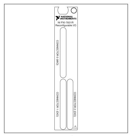
Figure B-1. NI PXI-7831R Connector Locations
